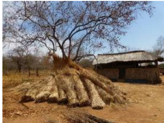
New grass bundles for roofing
